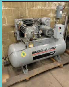
10-HP Ingersoll Rand T-30 Air Compressor
